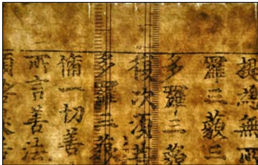
Figure 2. The paper of panel 6 of the Diamond Sutra viewed against light. Faint laid lines suggesting the usage of bamboo sieve attached to a 'floating' mould are visible in this picture.
