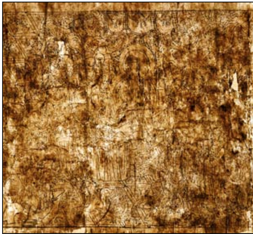
Figure 1. Fibre distribution in the paper of the Diamond Sutra 's frontispiece viewed on a light table. The print of the 'floating' mould with a textile sieve is visible in the paper structure.
